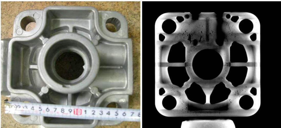
**Figure 5: Larger aluminium casting and a slice of the 225 kV cone beam CT scan: Artefacts due to lack of penetration**
