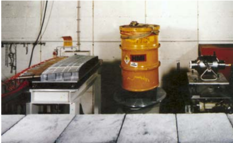
Fig. 2: First CT-Scanner of BAM
