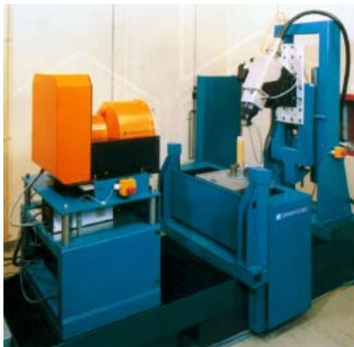
Fig. 5: First 3D-CT-Scanner (Sauerwein/BAM)
